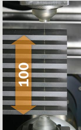
**Workpiece thickness 100mm**
