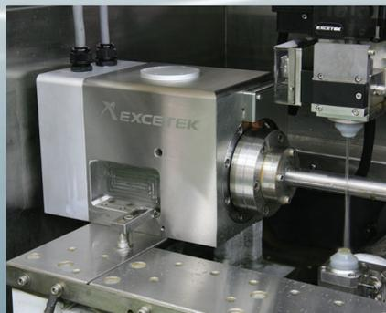
**PCD tool cutting module**
